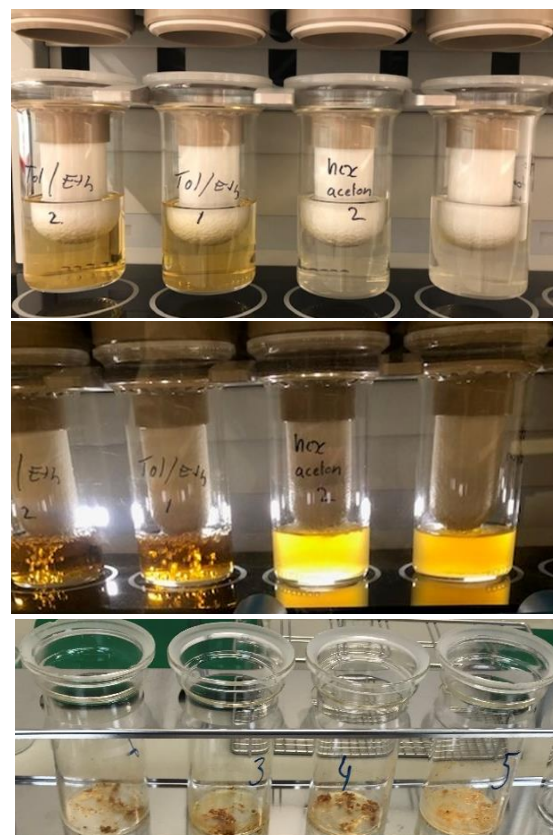
Figure 2 Pictures of the extract during the extraction process; top after adding solvent, middle after Twisselman and Soxhlet extraction and bottom after evaporation of the solvent. From left to right twice hexane : acetone and twice toluene ethanol.
