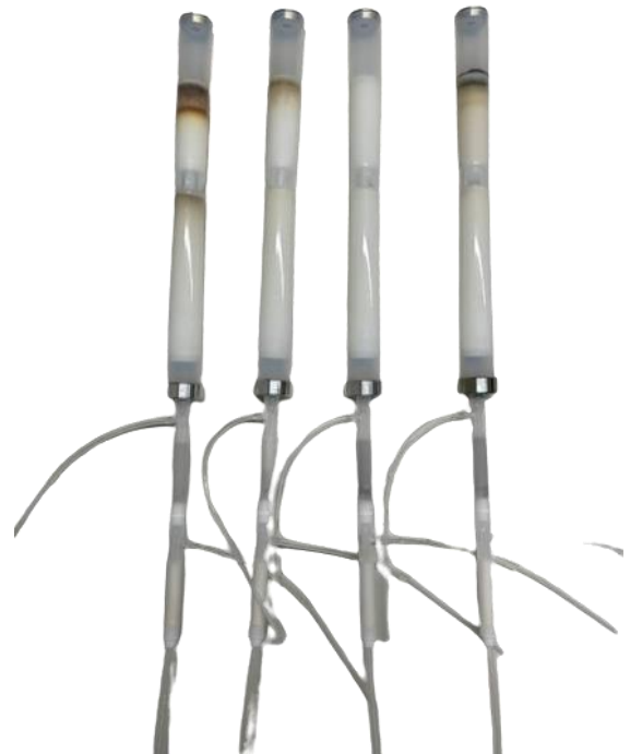
Figure 2 Column sets after clean-up procedure, from left to right sewage sludge, soil, ash and house dust.
